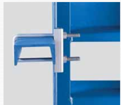
Channel Waler Clamp Mass 0.9kg Connects channel to form soldier.
